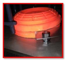
(f) When loading the clays be sure there are no tight spots in the carousel. Occasionally machines can suffer slight damage to the carousel.
