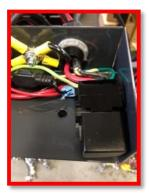
3. Inline fuse. Found inside electrical box. (7.5amp automotive type 2 prong fuse) https://www.youtube.com/watch?v=JZZmYQtybAE replacing fuse
